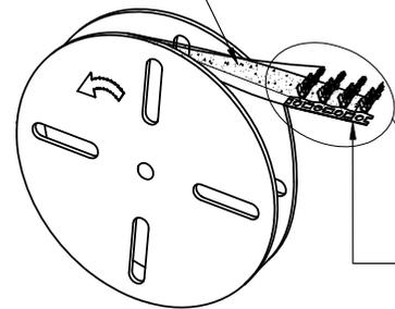
The terminal material belt is downward Wrap the thread with the foot facing upwards
